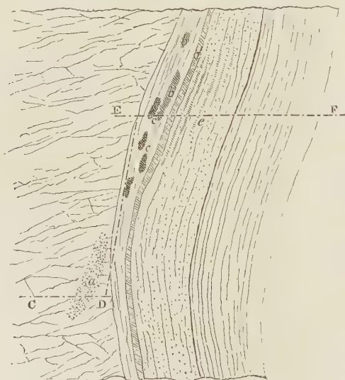
FIG. 84.—Copper ore deposit, Chessy; horizontal section on A B.
